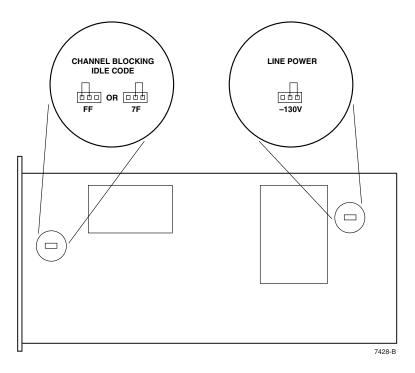
Figure 525-2. Placement of B1 RLX Jumpers
